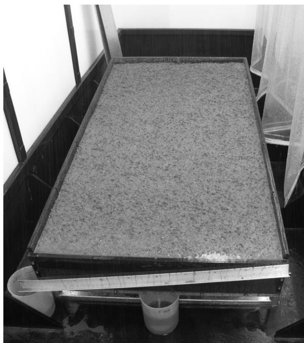
**Figure 3.** A silty loam was placed in a flume and subject to simulated rainfall.
